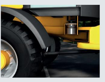
Stress on the driver is lowered due to optimized comfort, thereby increasing performance and driving safety. This is achieved by decoupling the dampers from the chassis and using Fabreeka hydraulic mounts for cabin suspension.
